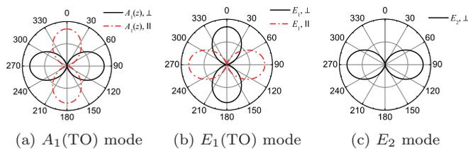
FIG. 4. (Color online) Calculated intensity polar patterns of the wurtzite modes for a nanowire oriented along  $\phi = 0^\circ$ . The  $E_2$  intensity is zero for parallel analysis ( $\parallel$ ). While the maximum intensity for the  $A_1$  mode is obtained in parallel configurations, the highest intensity of the  $E_1$  mode is achieved for crossed polarizations.
