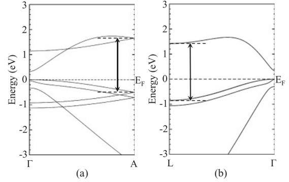
FIG. 8. *Ab initio* calculations of the electronic band structure of wurtzite (a) and zinc-blende (b) InAs along the directions  $\Gamma-A$  and  $\Gamma-L$ , respectively. The arrows denote the electronic transition energies at the corresponding symmetry points.
