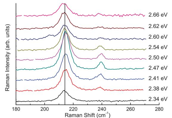
FIG. 9. (Color online) Series of Raman spectra from an InAs nanowire measured as a function of the laser energy. A resonance enhancement of the TO and LO mode is clearly visible.
