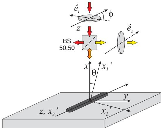
FIG. 1. (Color online) Schematic diagram of the experimental setup and the used coordinate systems ( $x, y, z$ ) and ( $x'_1, x'_2, x'_3$ ) in backscattering geometry.  $\hat{e}_i$  and  $\hat{e}_s$  are the incident and scattered light polarizations, respectively.
