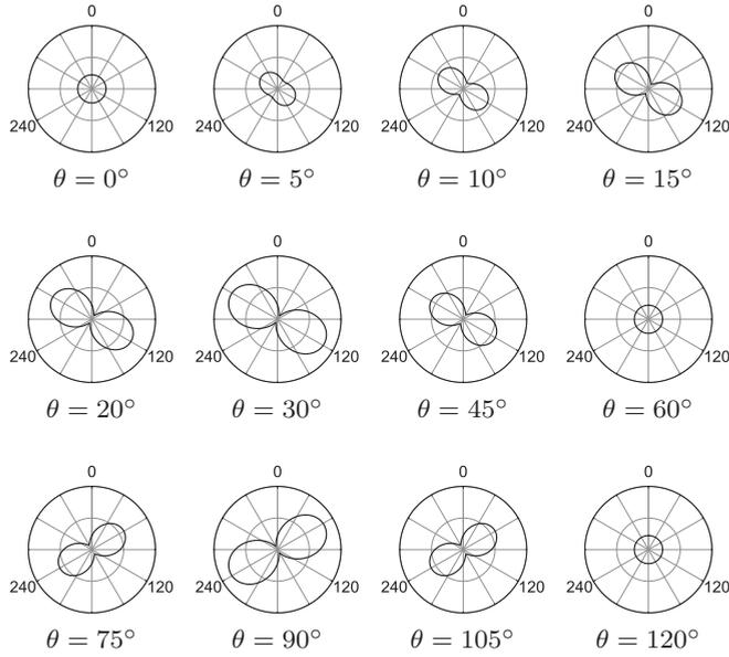
FIG. 3. Calculated intensity polar patterns of the TO mode under perpendicular analysis ( $\perp$ ) for different rotation angles  $\theta$  for a zinc-blende nanowire oriented along  $\phi = 0^\circ$ . The patterns present a periodicity of  $120^\circ$  and are independent of  $\phi$  for  $\theta = 0^\circ, 60^\circ, 120^\circ$ .
